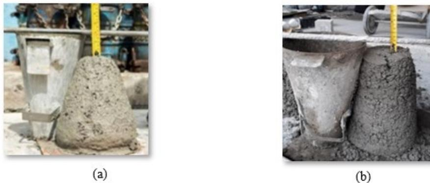
Figure 4: Slump test for (a) raw sawdust and (b) Epoxy sawdust
