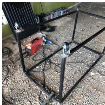
Figure 4: Welding process of the frame structure
