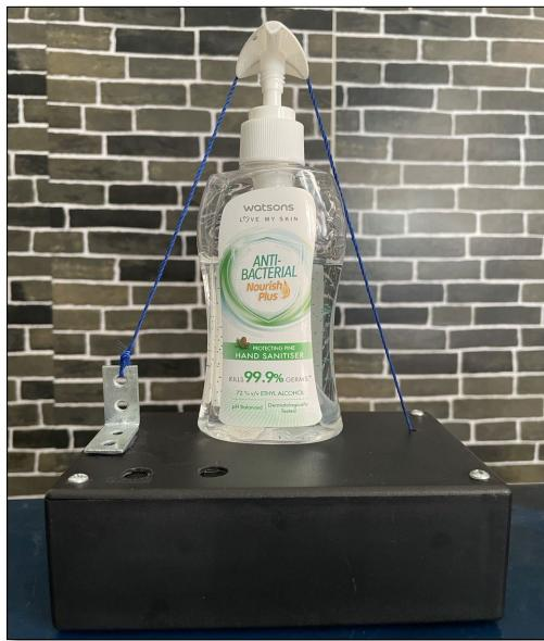
Figure 4 : Completed build of Touchless Hand Sanitizer
