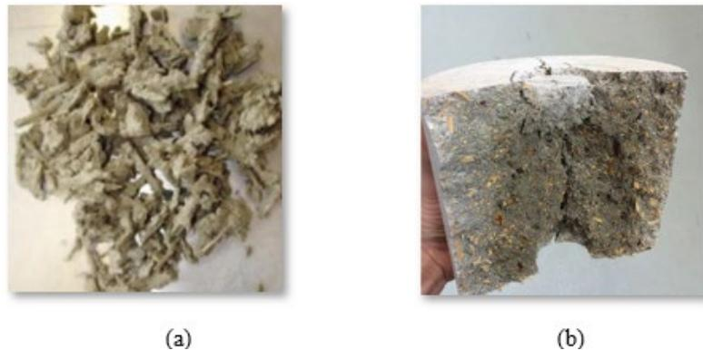
Figure 2: (a) Epoxy sawdust and (b) Epoxy sawdust cube mix sample
